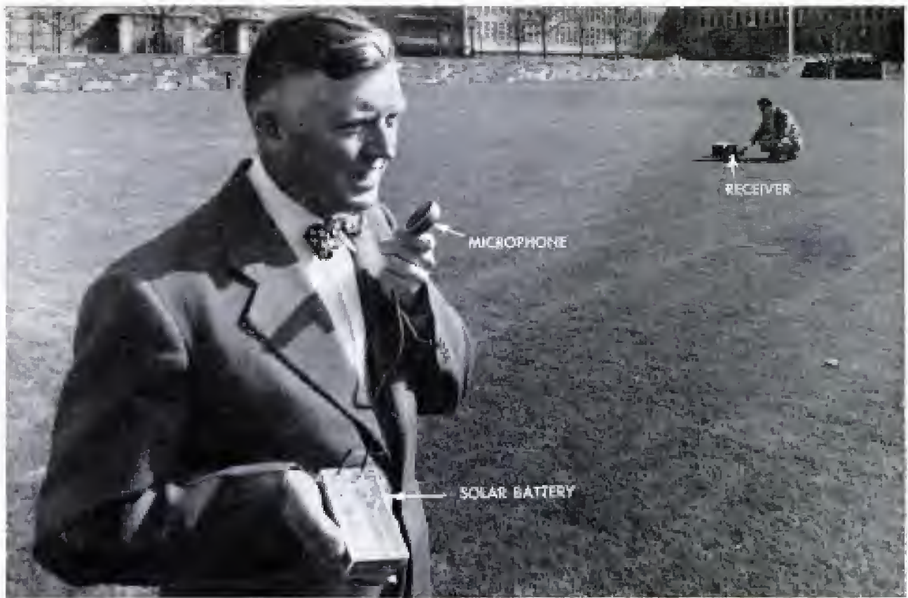
Solar battery powers pocket radio transmitter in demonstration. Some broadcasts have carried several miles
